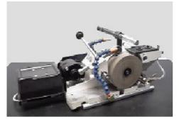
Model PGF Fixture is used for infeed and secondary operations of parts which have multiple diameters, gears, splines, etc. that require a relieved regulating roll, blade, etc. The Model PGF allows the operator easier access to the end of the part for ID grinding applications.
