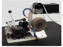
Our IGF Unit is designed for applications that require grinding the ID of parts closely concentric to the OD. Since concentricity tolerance of 0.000050" to 0.0001" have always been difficult to maintain, Unison offers users a simple solution.
